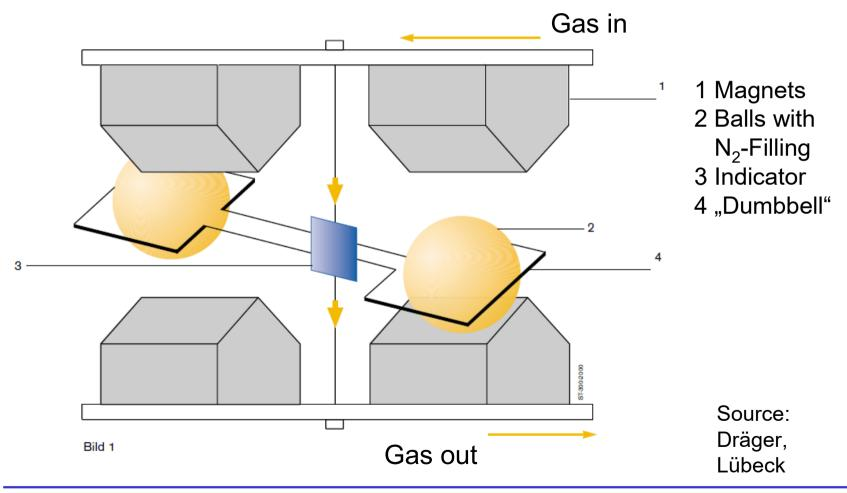
Standard Solution O<sub>2</sub>: by Paramagnetism: Magnetopneumatic Principle
