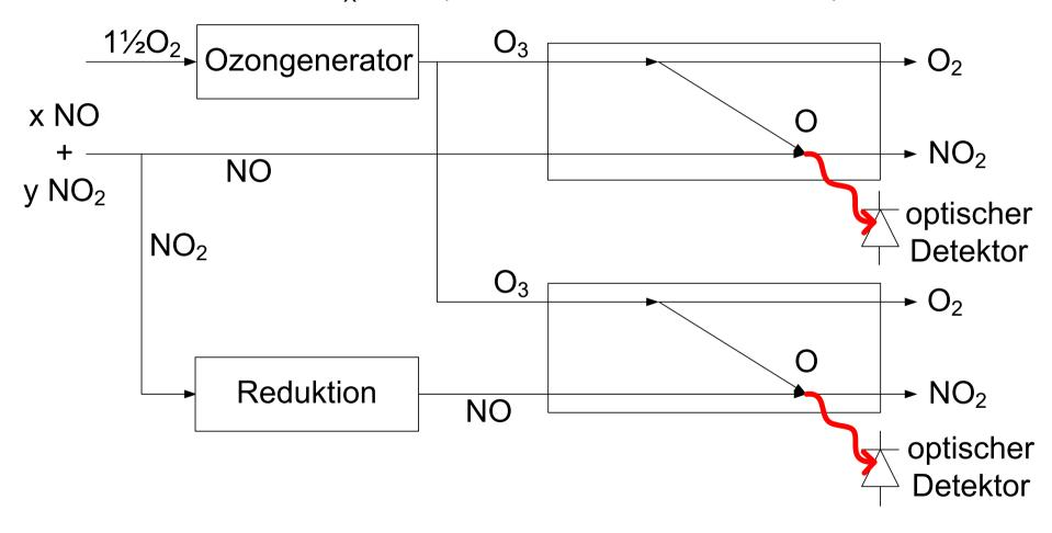
Standard Solution NO<sub>x</sub>: CLD (Chemiluminescence Detector)
